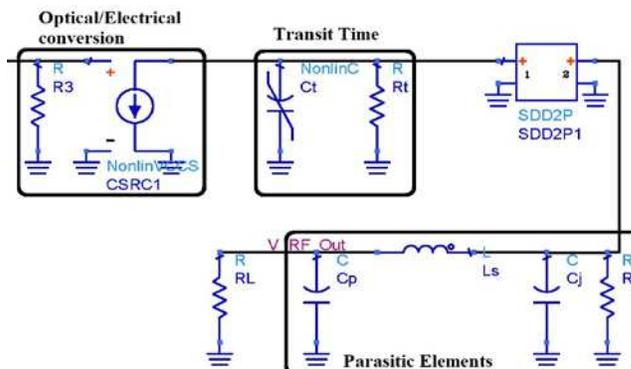
Fig. 4: A nonlinear equivalent circuit of a photodiode.
