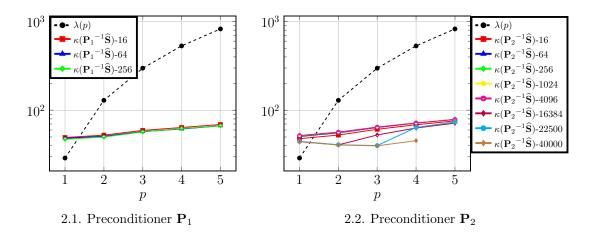
FIGURE 2. Condition number of the preconditioned system as function of p with 16, 64, 256, 1024, 4096 subdomains and n/N = 80
