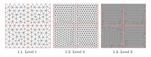
FIGURE 1. First three levels of refinements for unstructured triangular grids on a subdomain partition made of 4 squares.
