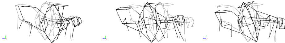
Figure 5: First 3 projected mode shapes for Pump 1.
