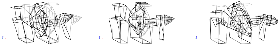
Figure 6: First 3 projected mode shapes for Pump 2.
