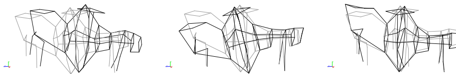
Figure 2: Pump 1: First three experimental mode shapes (Thick black line).
