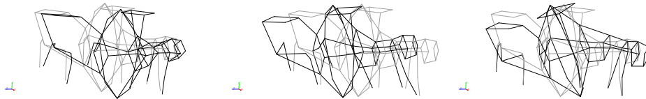
Figure 5: First 3 projected mode shapes for Pump 1.
