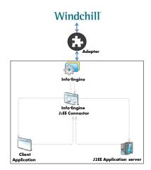
Fig. 3. The info\*Engine based architecture
