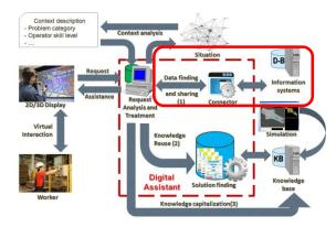
Fig. 2. Functional architecture of the digital factory assistant
