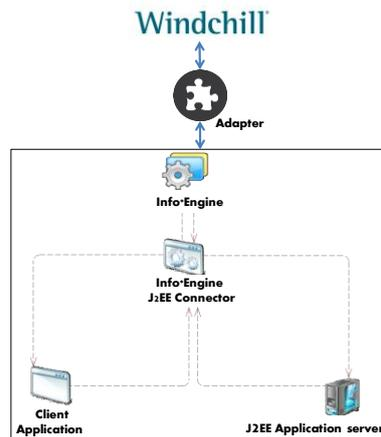
Fig. 3. The info\*Engine based architecture
