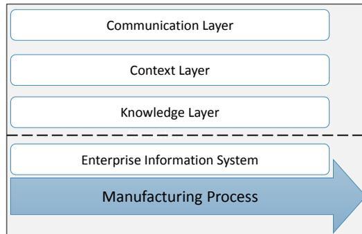
**Fig. 1.** Conceptual architecture of the Digital Factory Assistant
