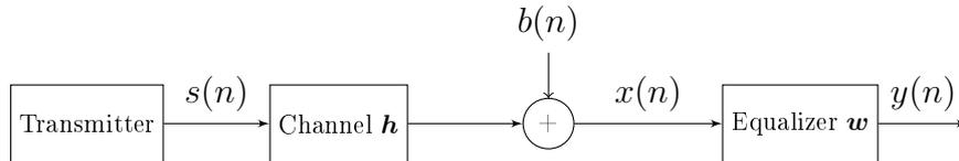
Figure 1: Basic scheme of a blind equalization system
