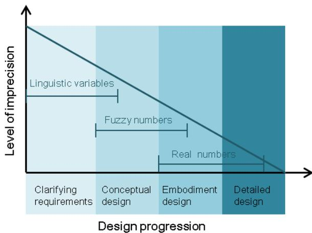
Figure 3: Design stages versus imprecision level [AO1].
