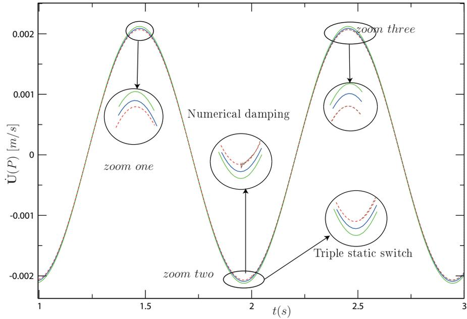
(b) Velocities: comparison between the numerical damping method and the triple static switch method
