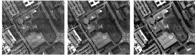
Fig. 2. ROSIS dataset: Detail of band 1 of the original image(left) and the reconstructed images using 4 components from the PCA (center) and NLPCA (right) approaches, respectively.
