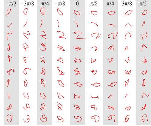
Fig. 6. Trajectories generated by the network for different rotation angles. Digits on gray background correspond to rotation angles which were presented to the network during training (only one trajectory for each (digit, rotation angle) pair was provided for training). Other trajectories show the generalization capabilities of the network.
