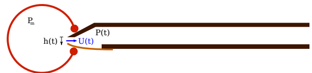
Figure 1: Schematics of the clarinet and variables used in the physical model.
