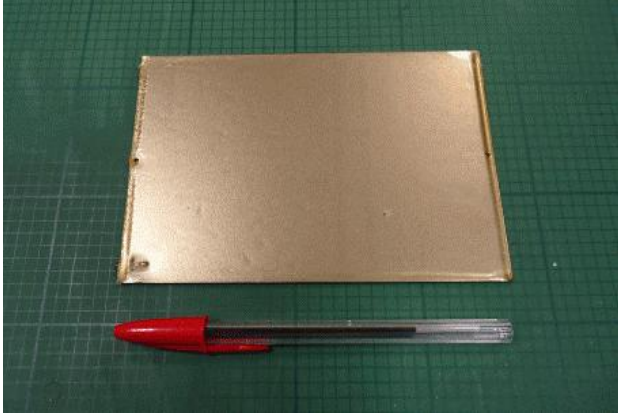
Fig. 1. Tested 90µm coated steel plate (15cm x 9cm)
