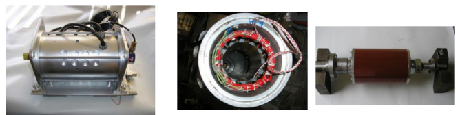
Fig.12 : Machine Synchrone MS 10p-12s
