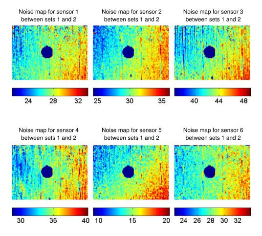
This bias could be due to some vibrations generated by the rotation of the mirror in the camera that could induce slight movements of the sensors from their initial positions. It has to be noted that the shift of the average value does not affect strains (as strains are displacement gradients) but does affect the acceleration.
