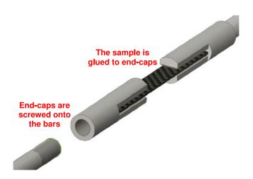
$\textbf{Fig. 12} \quad \text{Attachment of the sample to the SHPB set up} \\$
