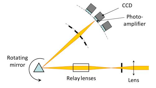
and triggering issues, the interframe time was limited to 3.3 µs (i.e., a frequency of acquisition of 300,000 fps).
