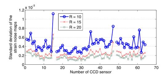
**Fig. 6** Level of strain rate noise plotted for each sensor
