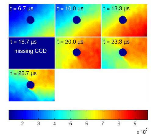
**Fig. 18**  $a_x$  maps (colormap in m·s<sup>-2</sup>) (test 2, tensile direction: horizontal, field of view:  $20 \times 16$  mm)
