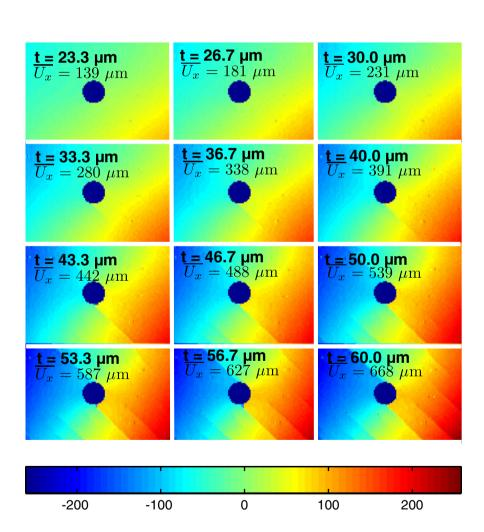
**Fig. 11**  $\varepsilon_{xx}$  maps (test 1, tensile direction: horizontal, field of view:  $20 \times 16$  mm)
