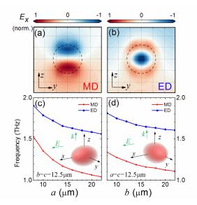
Fig. 2. (a) FDTD simulated MD (1.21 THz) and (b) ED (1.66 THz) modes in a TiO<sub>2</sub> sphere ( $\varepsilon$  = 100, radius  $r = 12.5 \,\mu$ m); the x-polarized incident EM wave propagates along the z-axis. The color represents the electric field ( $E_x$ ) normalized to the maximum field within the sphere. (c) and (d) Resonance frequencies of the MD and ED modes in an elliptical resonator.
