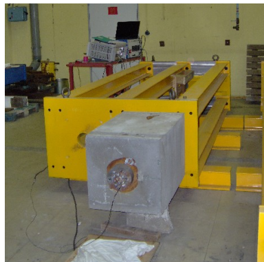
Figure 5. 5 m bench for cement grouted 7-wire strand prestressed at 80% of the ultimate strength
