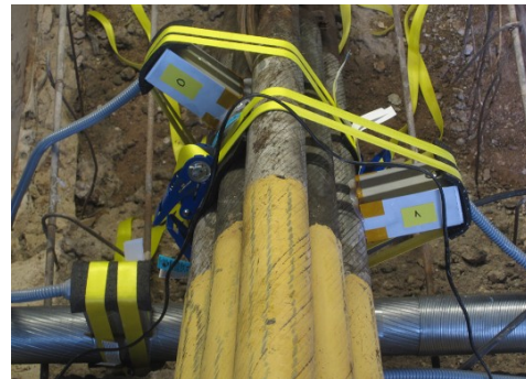
Figure 8. Schematic representation of the monitoring equipment tested in Mettlach and photo of three installed devices (two on the loaded ropes and one device on an unloaded similar rope located below the loaded ropes)
