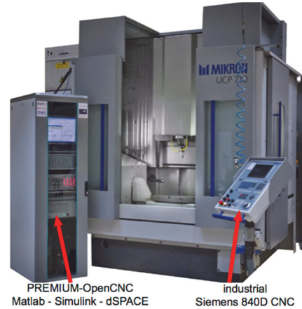
Fig. 4: 5-axis high speed milling machine with the PREMIUM-OpenCNC and the Siemens 840D CNC
