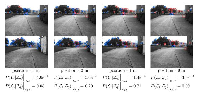
Figure 8: Demonstration of matched features and posterior probability values as a location which matches the query is approached. The query image is repeated in the top row, with four other locations preceding a match to the query shown in the second row. Matched visual words are marked by circles, while unmatched visual words are marked by x's. The resulting match probabilities are shown below each image pair.
