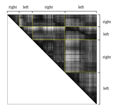
Figure 20: The confusion matrix when comparing differences (SAD) between all the images of the street sequence, with lighter pixels indicating larger differences. Highlighted lines indicate the start of each new traverse down the street. Only half the matrix is shown because of symmetry. The SeqSLAM algorithm [Milford, 2013] searches for diagonals of low difference values in the matrix.
