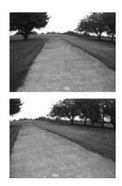
Figure 12: Example of a significant perspective changes in the Begbroke dataset. These perspective changes introduce difficulties for algorithms which rely on direct image comparisons, such as SeqSLAM.
