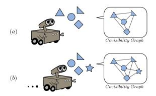
Figure 1: As the robot moves, it makes observations, detects landmarks, and notes which ones were seen together in a graph structure. Here you can see a simple example of two steps as a robot moves forward through the environment, and the resulting covisibility graph.
