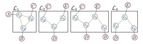
Figure 3: Given the query  $\mathcal{Z}_q = \{C, D, E\}$  and covisibility map  $\mathcal{M}_k$  (both shown in Fig. 2), will produce four virtual locations,  $\mathcal{L}_1$ ,  $\mathcal{L}_2$ ,  $\mathcal{L}_3 \& \mathcal{L}_4$ .
