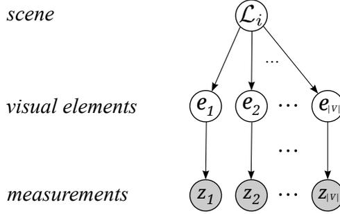
Figure 4: Graph of the observation model, with observed variables shaded in gray. A location consists of a set of visual elements  $e_n$ , which are then observed by an imperfect sensor, giving measurements  $z_n$ . The possible set of visual elements is defined by a visual dictionary of size  $|\mathcal{V}|$ , and visual features  $e_n$  and  $z_n$  take on boolean values based on existence or observation respectively.
