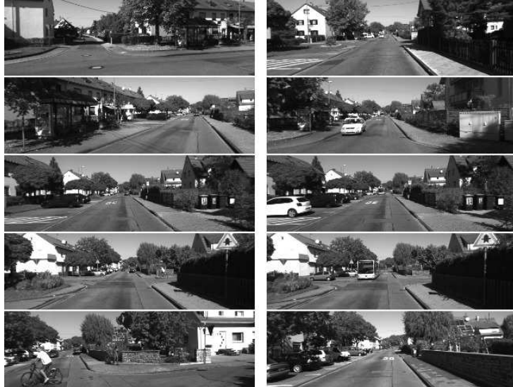
Figure 16: Example of a loop-closure sequence which is shorter than the sequence length used in the SeqSLAM algorithm, resulting in relatively low scores and therefore missed loop-closures. The left column shows the image sequence from one pass, and the right shows the image sequence from a second pass (only a subset of images from the sequence are shown).
