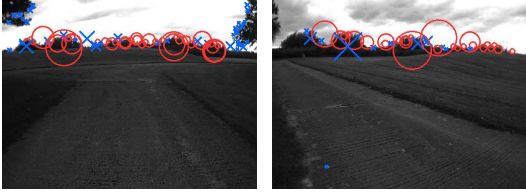
Figure 7: Examples of images from the Begbroke sequence which correspond to the regions of confusion in first matrix of Figure 6, due to their non-discriminative appearance. The images contain many matched visual words (marked with circles), despite depicting different locations. However, these locations tend to produce low matching probabilities regardless, which indicates a low confidence due to common appearance.
