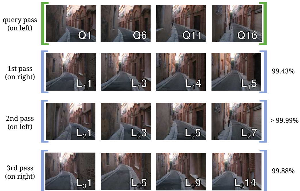
Figure 19: Given the query shown in the top row, the most probable virtual locations from three separate traverses of a street are shown (only four images are displayed per location for clarity). Both the query and the second pass are traversed on the left side of the street, while the first and third passes are traversed on the right side. The images collected from the query were generated from a much slower and erratic traverse (including backtracking), resulting in more images, but representing the same traverse. Images are labeled with their corresponding number in the retrieved sequence.
