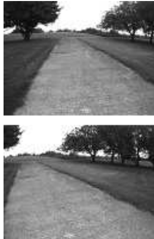
Figure 12: Example of a significant perspective changes in the Begbroke dataset. These perspective changes introduce difficulties for algorithms which rely on direct image comparisons, such as SeqSLAM.
