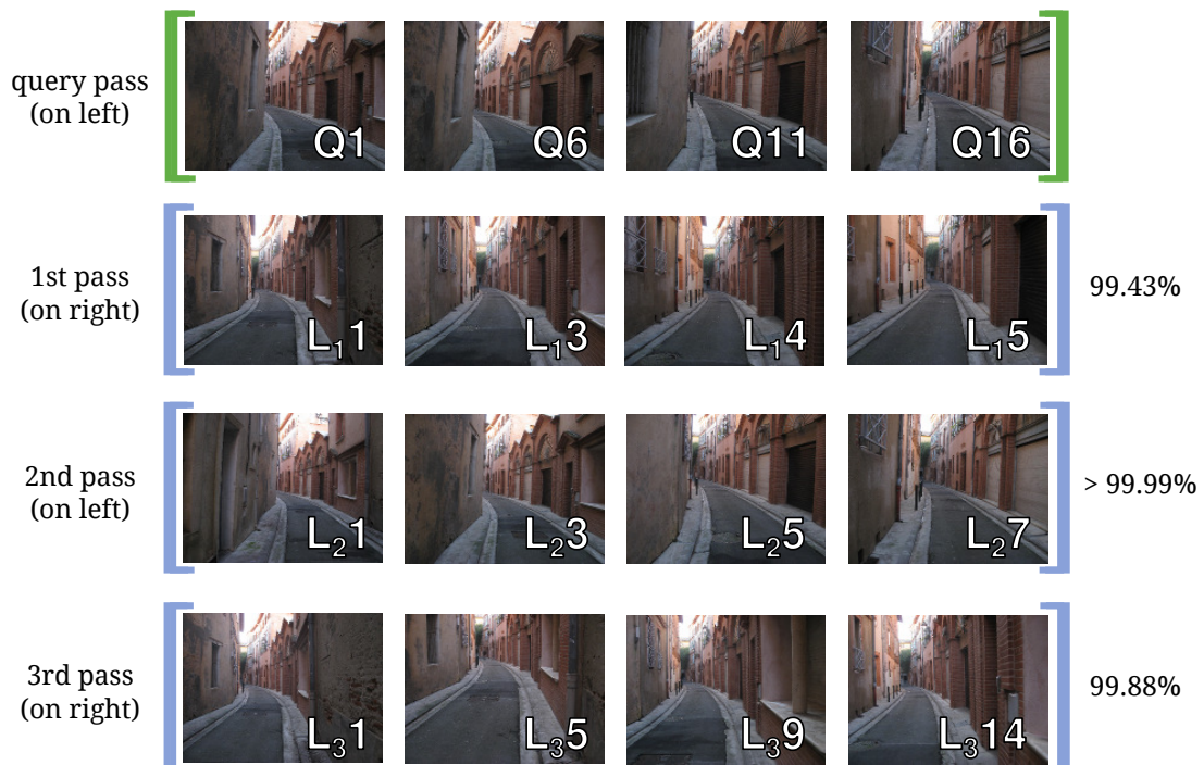
Figure 19: Given the query shown in green, the most probable virtual locations from three separate traverses of a street are shown (with only four images displayed per location for clarity). Both the query and the second pass are traversed on the left side of the street, while the first and third passes are traversed on the right side. In addition, the images collected from the query were generated from a much slower and erratic traverse (including backtracking), resulting in more images representing the same traverse yet poses no problems for the system.
