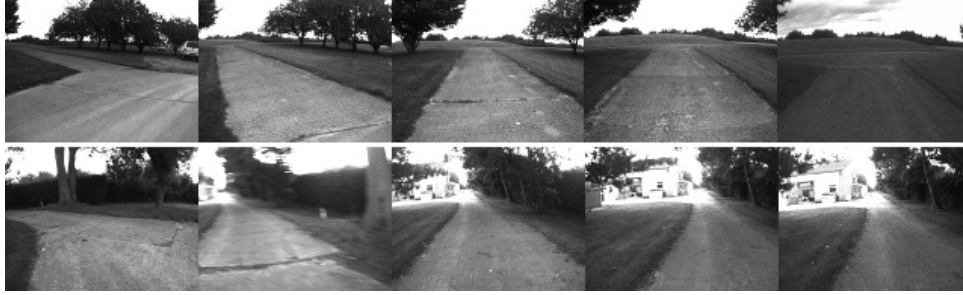
Figure 11: A subset of images from a false positive sequence match example from SeqSLAM on the Begbroke dataset.
