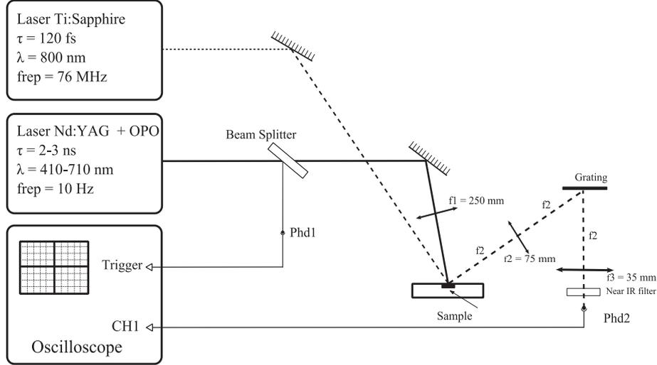
**Figure 1.** All optical single-shot pump-probe reflectivity measurement set-up.
