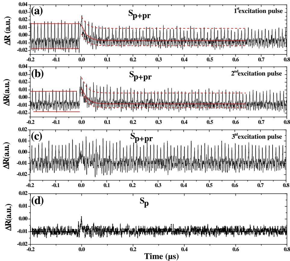
**Figure 5.** Reflectivity evolution upon pulsed excitation ( $\tau = 3$  ns,  $\lambda = 532$  nm,  $E = 5.7 \cdot 10^{-6}$  mJ  $\mu\text{m}^{-2}$ ). The photo-excited area is gradually switched from of the  $\beta$ - to  $\lambda$ - phase transition for (a) the 1st, (b) the 2nd and (c) the 3rd excitation pulses. (d) Signal recorded without probe beam upon the 4th pump excitation.
