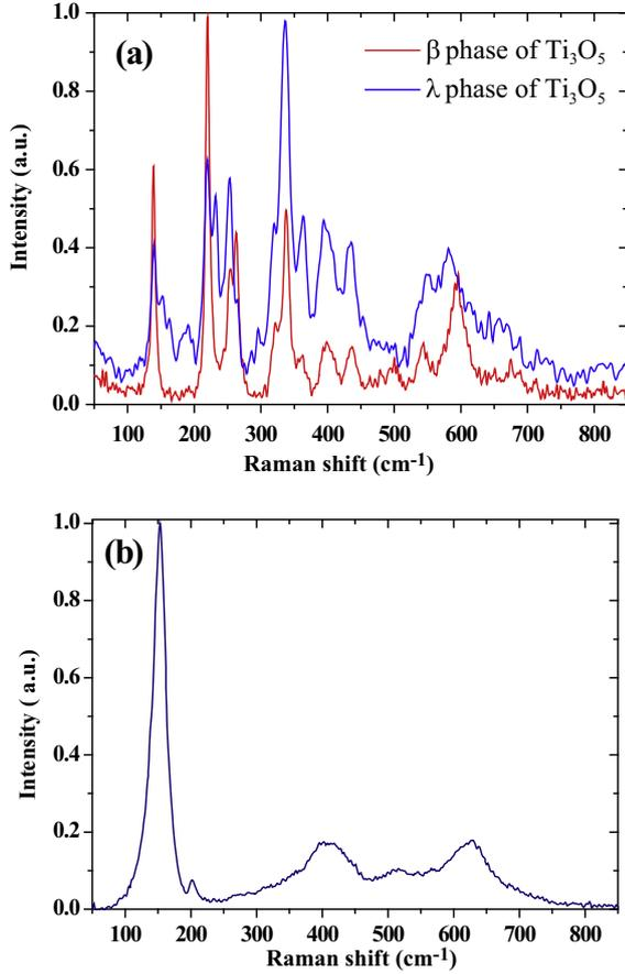
**Figure 3.** (a) Raman spectra of the sample in the  $\lambda$ - and  $\beta$ - $\text{Ti}_3\text{O}_5$  phases. (b) Raman spectrum of the  $\lambda$ - $\text{Ti}_3\text{O}_5$  nanoparticles after QCW laser excitation ( $I = 2.8 \cdot 10^{-3} \text{ mW } \mu\text{m}^{-2}$ ). This spectrum resembles the one recorded for  $\text{TiO}_2$  nanoparticles.
