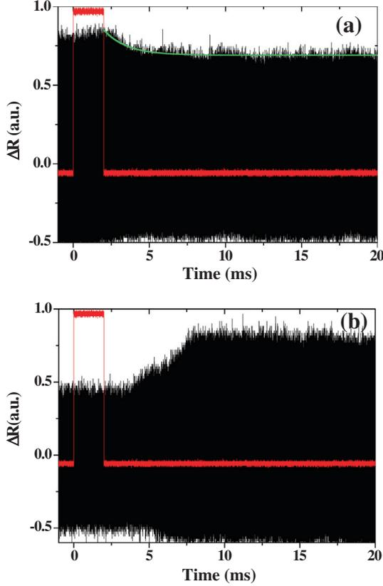
**Figure 6.** (a) Reflectivity evolution upon application of QCW laser pulse ( $\tau = 2$  ms,  $\lambda = 532$  nm,  $I = 2.4 \cdot 10^{-3}$  mW  $\mu\text{m}^{-2}$ ). The sample is switched from  $\lambda$ - to  $\beta$ -Ti<sub>3</sub>O<sub>5</sub>. (b) Reflectivity evolution upon application of QCW laser pulse ( $\tau = 2$  ms,  $\lambda = 532$  nm,  $I = 2.8 \cdot 10^{-3}$  mW  $\mu\text{m}^{-2}$ ).
