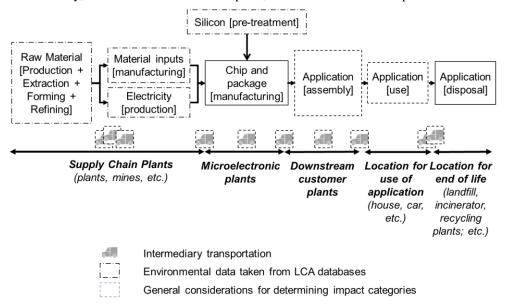
Fig. 1. General phases in a component lifecycle.
