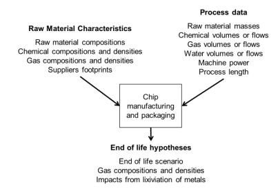
Fig. 2. General phases in a component lifecycle.
