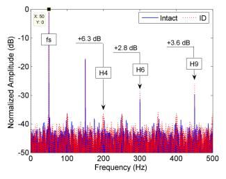
Fig. 8. Stray flux spectra: intact – ID for no-load generator.
