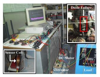
Fig. 5. Laboratory test bench.
