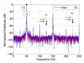
Fig. 6. Output voltage spectra: intact – ID for no-load generator.
