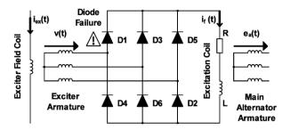
Fig. 2. Rotating Diodes bridge.
