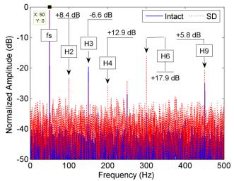
Fig. 13. Stray flux: intact – SD for balanced resistive full-load.
