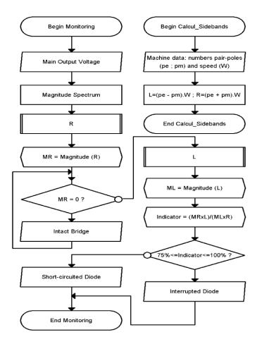
Fig. 14. Monitoring algorithm based on output voltage.
