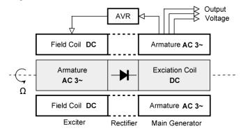
Fig. 1. Typical architecture of brushless synchronous generators.
