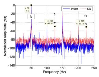
Fig. 7. Output voltage spectra: intact – SD for no-load generator.
