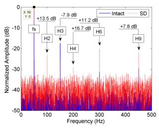
Fig. 9. Stray flux spectra: intact – SD for no-load generator. For both conditions, these spectra are characterized by an amplitude rise, observed especially for the 4th, the 6th, and the 9th harmonics. However, this augmentation is much accentuated when the generator runs under SD condition. In addition, for this particular fault condition, a clear increase in
