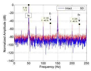
Fig. 11. Output voltage spectra: intact - SD for balanced resistive full-load.
