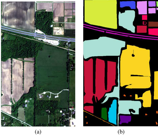
Figure 3: Indian Pines 2010 SpecTIR data. (a) RGB composition and (b) Ground truth (for color legend, see Tab. 2). Unlabeled samples are in black.
