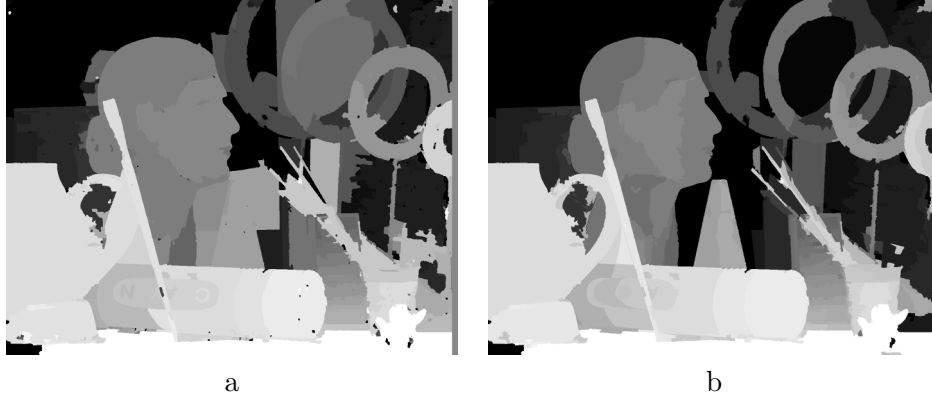
Figure 2. Comparison between (a) brute and (b) rectified regional disparities which handle semi-occluded regions on the coarse partition of Middlebury Art image [13].
