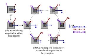
Fig. 3: POEM feature extraction for one pixel p. In (s3), the algorithm considers the length of vectors.
