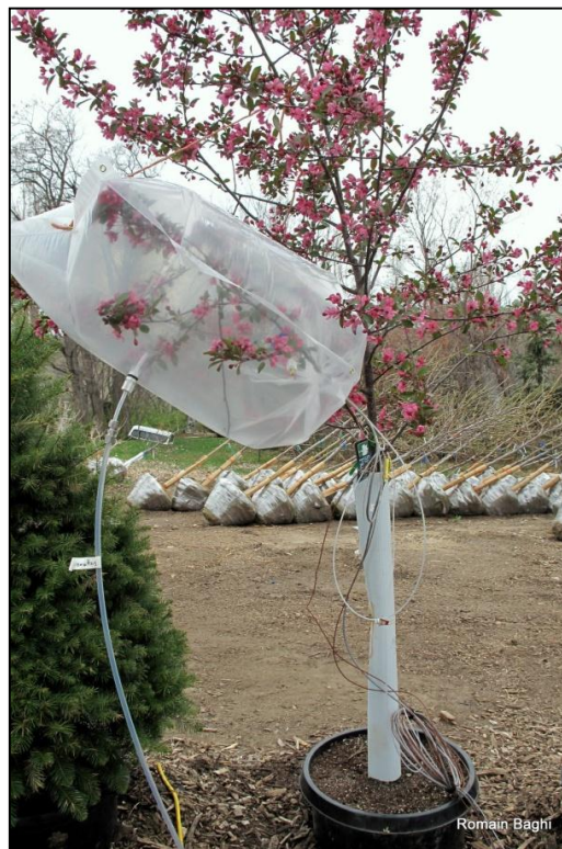
Fig. 1. Branch enclosure experiment setup on a crabapple tree during its flowering period.
