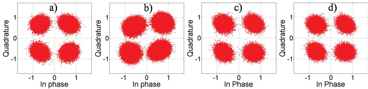
Figure 3. Experimental QPSK constellations at 12 dB OSNR: a) without IQ imbalance, b) with IQ imbalance of 15°, c) recovered using the GSOP method, d) recovered using the proposed MSEM method.
