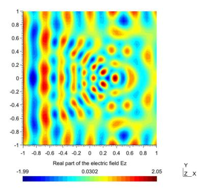
Fig. 5.4: Real part of the electric field for the scattering of a plane wave in a multi-layer domain.
