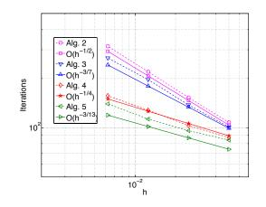
Fig. 5.3: Asymptotic behavior of the iteration numbers from Table 5.5 as a function of the mesh size h.
