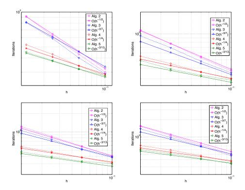
Fig. 5.1: Asymptotic behavior of the iteration numbers from Table 5.3 as a function of the mesh size h for the DG- $\mathbb{P}_1$ , DG- $\mathbb{P}_2$ , DG- $\mathbb{P}_3$ , and DG- $\mathbb{P}_4$  discretizations.
