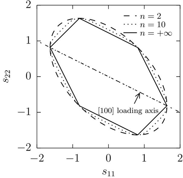
Figure 1: Section of regularized Schmid yield functions and the Bishop-Hill polyhedron [34] in the deviatoric stress plane  $(s_{11}, s_{22})$ . The axial loading corresponding to the [100] crystalline direction is indicated.
