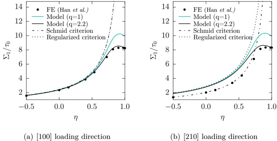
Figure 4: Normalized yield stress  $\Sigma_1/\tau_0$  as a function of the axisymmetric loading parameter  $\eta = \eta_2 = \eta_3$  for porous FCC single crystals. The yield criterion using a quadratic regularized Schmid law (26) (solid lines) is compared to unit-cell computations reported in [28] (points). Porosity  $f = 1\%$ . The yield stress of the bulk single crystal according to the standard and quadratic regularized Schmid law is indicated (dashed and dotted lines).
