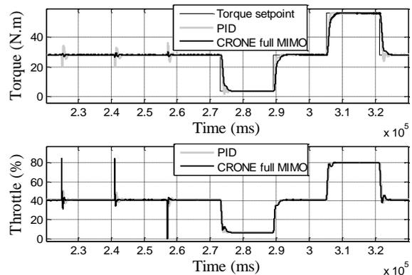
**Fig. 9:** Torque set-point tracking and throttle control effort
