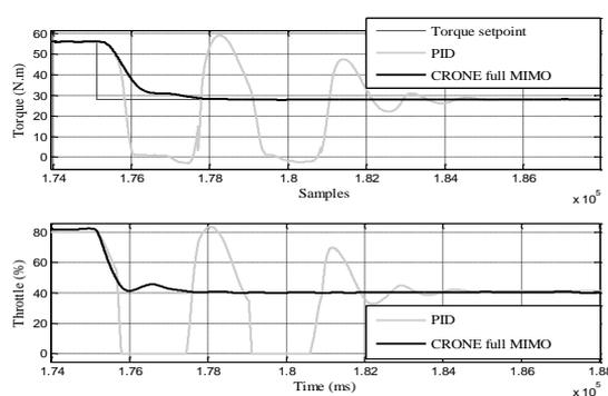
**Fig. 10:** Robustness problem during a torque step
