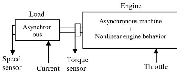
**Fig. 1:** Test-bed configuration
