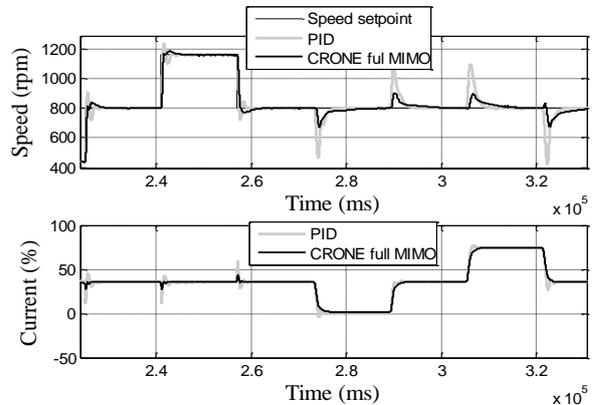
**Fig. 8:** Speed set-points tracking and current control effort
