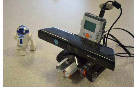
Figure 5. Our system composed by a Lego Mindstorm vehicle and a Kinect
