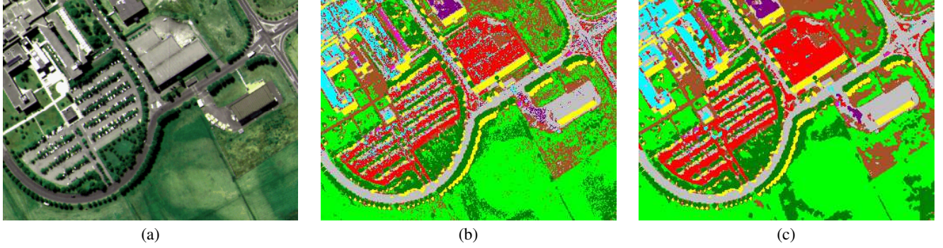
Fig. 1. (a) RGB color composition for the University area , thematic map obtained with (b) p\mathcal{GP}_1 and (c) the p\mathcal{GPMRF} .
