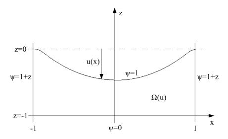
FIGURE 1. Idealized electrostatic MEMS device.
