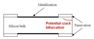
Fig. 12. Schematic crack propagation which bifurcated through silicon.
