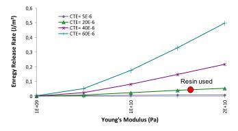
Fig. 15. Variation of nergy release rate G (J/m<sup>2</sup>) versus Young's modulus (Pa) of resin considering different CTEs (C<sup>-1</sup>) of resin (electrothermal load, crack length = 30  $\mu$ m, distance = 10  $\mu$ m).
