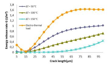
Fig. 8. Variation of energy release rate G (J/m<sup>2</sup>) versus crack length ( $\mu$ m) for different temperatures.
