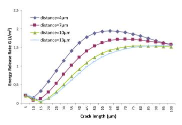
Fig. 9. Variation of energy release rate G (J/m<sup>2</sup>) versus crack length ( $\mu$ m) for different distance between crack and Si/passivation interface (electrothermal load).
