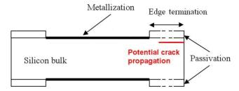
Fig. 10. Schematic variation of the edge termination length.
