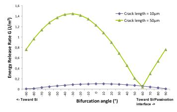
Fig. 13. Variation of energy release rate G (J/m<sup>2</sup>) versus bifurcation angle (°) for two crack lengths of 10 and 50  $\mu$ m (electrothermal load, distance = 10  $\mu$ m).
