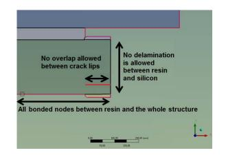
Fig. 6. Numerical contact models applied on the structure.
