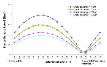
Fig. 14. Energy release rate G (J/m<sup>2</sup>) versus bifurcation angle (°) for different distances between crack and Si/passivation interface (electrothermal load, crack length = 40  $\mu$ m).
