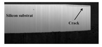
Fig. 7. Example of straight crack propagation in silicon and its position from passivation after thermal cycling test.
