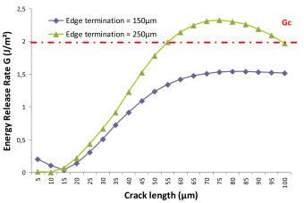
Fig. 11. Variation of energy release rate G (J/m<sup>2</sup>) versus crack length ( $\mu$ m) for two different junction edge termination sizes (electrothermal load, distance = 10  $\mu$ m).
