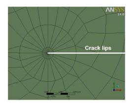
Fig. 5. Refined meshing around crack tip and crack lips.
