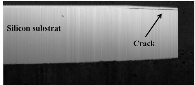
Fig. 7. Example of straight crack propagation in silicon and its position from passivation after thermal cycling test.
