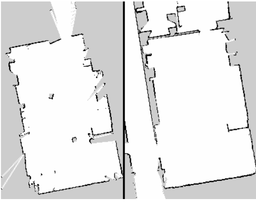
Fig. 2. A Static Map after the first run of the robot (left), and after several runs (right).
