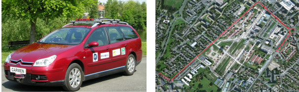
(a) CARMEN vehicle. Velodyne is installed on top (b) Trajectory of the Experiment (Red line)
