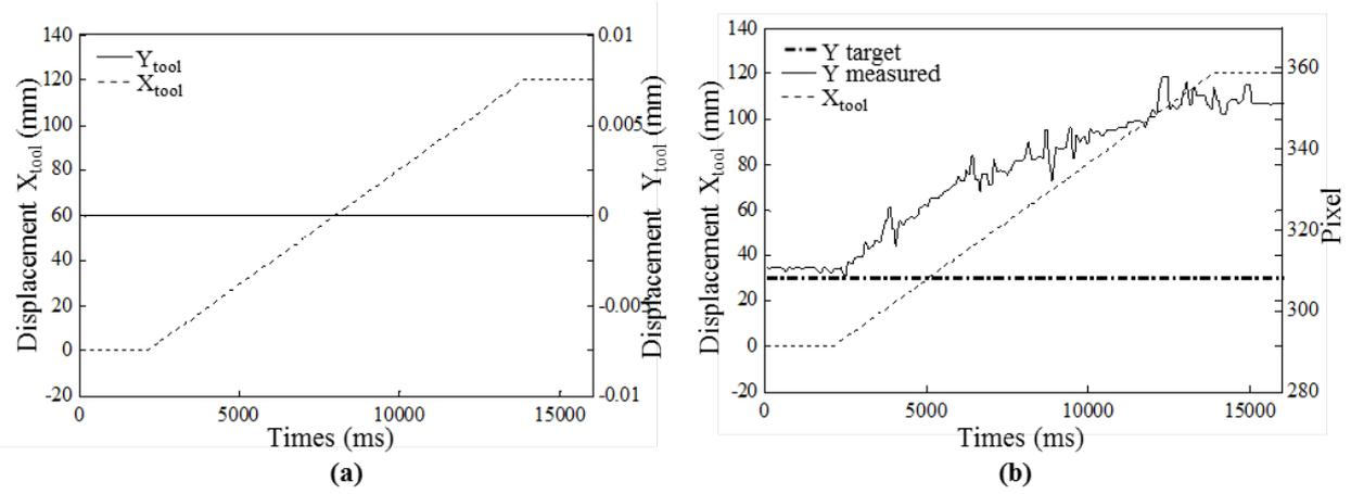
Figure 23: Edge monitoring during  $x$ -axis motion
