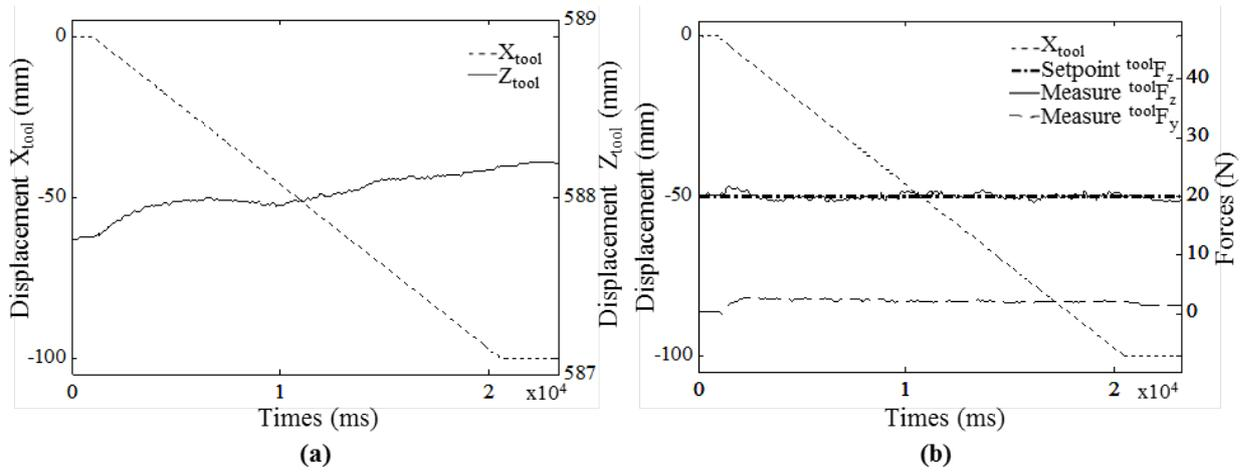
Figure 19: Compacting strength with force control during motion
