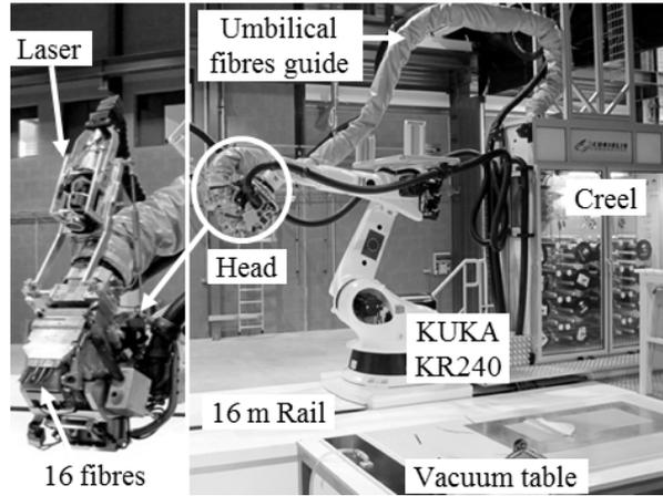
Figure 1: Robotic cell for Automated Fibre Placement
