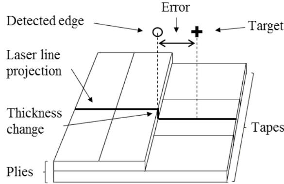
Figure 8: Thickness detection
