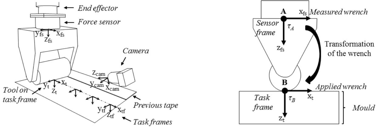
Figure 6: Task frame and transformation of moment
