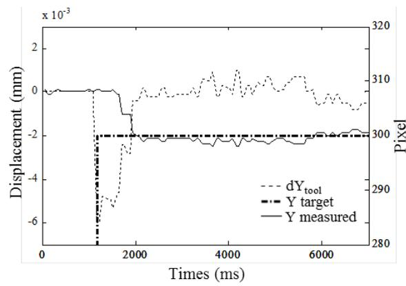
Figure 22: Visual servoing step response
