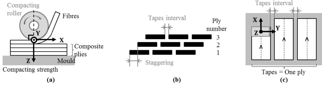
Figure 2: Laying-up process: a) Side view; b) Front view; c) Top view
