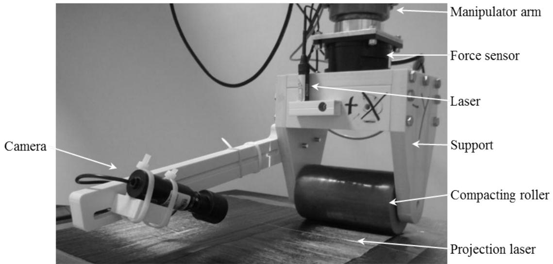
Figure 16: Camera, laser beam setup on the FPT
