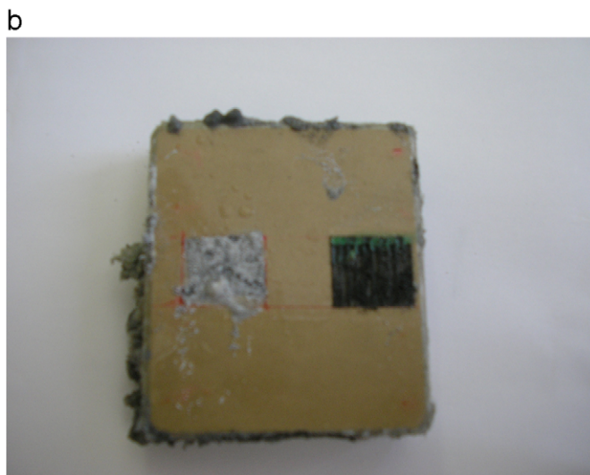
Fig. 8. Evolution of the corrosion in a salt-spray room of a LSMT and an as-received ZE41 alloy: (a) after 2 h of exposure and (b) after 131 h.
