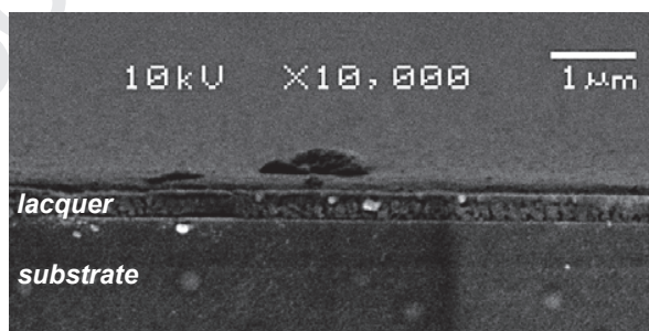
Fig. 3. Lacquer coating on a cleaved substrate (scanning electron microscope picture).
