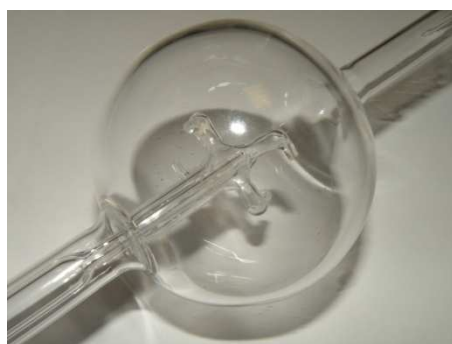
Figure 5. Photograph of the fused silica JSR used by the Nancy team showing the injection cross and the outlet tube.
