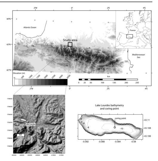
raised bog. Lake Lourdes was cored with an Uwitec gravity corer (6.3 cm in diameter) and 10 overlapping 3 m-long sections were retrieved from 3 boreholes at the deepest part of the lake (Fig. 1).
