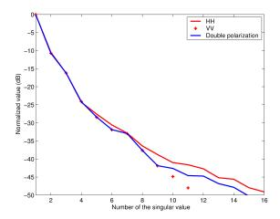
Fig. 8. Singular values of the interference matrices for single polarization (HH and VV) and dual polarization for simulated data. The ranks of the interference subspaces are chosen to be  $D_J^H = D_J^V = 10$  for single polarization and  $D_J = 10$  for dual polarization.
