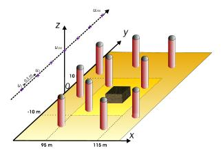
Fig. 6. Scene configuration for the simulated data. A PC box of size  $(2m \times 1.5m \times 1m)$  over a PC flat ground and located at position (108, -1)m is placed in a forest of dielectric trunks, for an transmitted signal with center frequency of 400MHz and with bandwidth of 100MHz. The attenuation due to the canopy is also taken into account.
