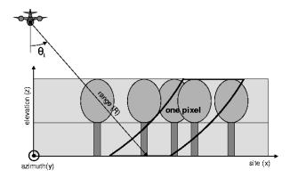
Fig. 2. Definition of the incidence angles  $(\theta_i, \varphi_i)$ .
