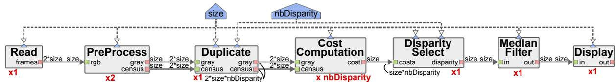
Figure 4: PiSDF graph of the stereo matching application
