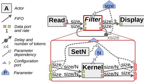
Figure 2: An Example of a PiSDF Model
