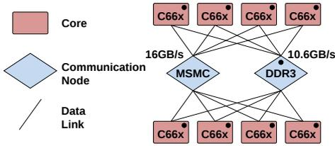
Figure 3: An Example of a S-LAM Model
