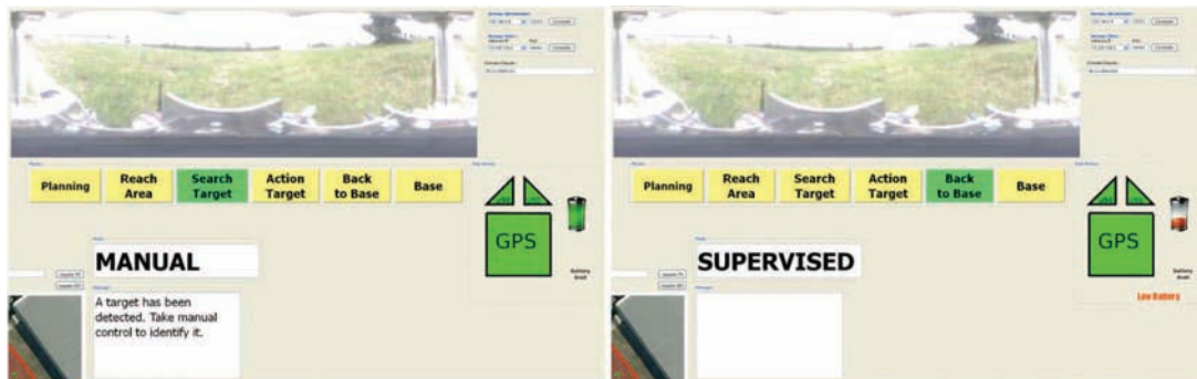
Figure 2. The upper panel shows the graphical user interface (GUI) before the failure, and the bottom panel displays the GUI with the low-battery event: The mission segment changes from “Search target” to “Back to base,” the battery icon turns from green to orange with an associated message, and the message on the interactive panel disappears.
