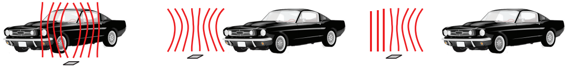
Figure S1. From right to left: perturbation of Earth's magnetic field (red lines) produced by a vehicle approaching and passing through the detection zone of a magnetic sensor (gray rectangle).
