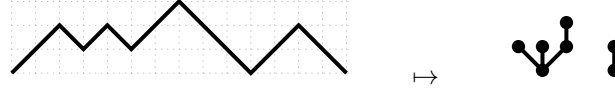
Fig. 3: The bijection from Dyck paths to plane forests. Here the Dyck path is rotated clockwise by an angle of 45^\circ . A pair of matching up step and down step corresponds to a vertex.
